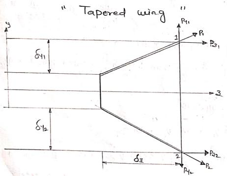
Pz1 and Pz2 are the components in the z direction of the axial loads P1 and P2 in the flangs and Py1 and Py2 are the components parallel to y axis.
