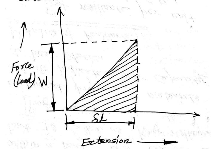
Strain energy stored in the bour = Work done by the load 1/2. W.S.L Where, A => Area E=> Modulus of Elasticity 1=) length of bar => Volume of bar T=> stress, be the proof stress
