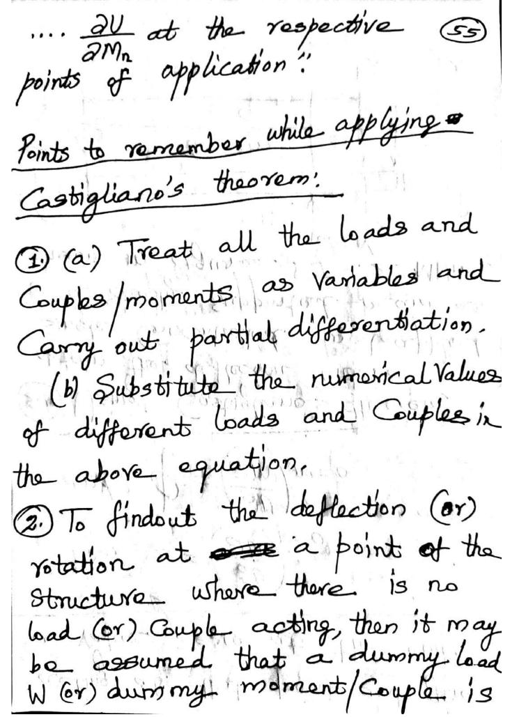
acting at that point an a value zero at the and give i.e.,  $\chi = \left(\frac{\partial U}{\partial W}\right)_{W=1}$ sing Castigliano's theorem the deflection under a Single Concentrated load applies to a Simply supported beam
