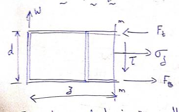
The direct load in the planges are found by considering a length 3 of the beam.
