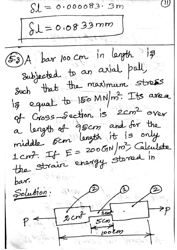
Maximum stress in portion of I cm Gross-Section, 0,= 150 MN/m2 Maximum stress in portion of 2cm2 Cross- Section, 02 = 75 MN/m2 WKT, O, A, = 02 Az 150X1X104 = 02 X 2X10 102 = 150 = 75 MN/m2 Strain energy stored in the bar, U= 0,2A,1, + 02A212 U= (150×106) x (1-×10-4) x (5/100) 2x (200x (09) (75×106)2×(2×104)× [95/100]
