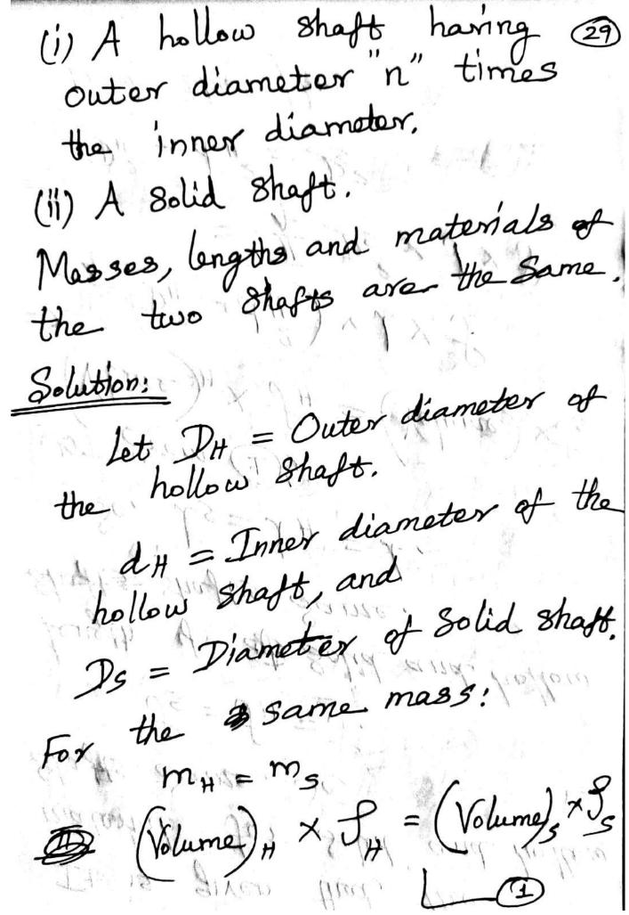
It is given that, the material for solid and hollow Shafts Same. So,  $f_g = f_H = f.$ Length of Solid and hollow shafts Shafts Same. So,  $L_s = L_H = L_s$ WKIT from (1),
