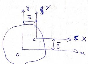
The moment of inertia of an area about an any through o is regulated to the moment of inertia of the area about a possible anis through the centroid C + the area multipled through the centroid C + the area multipled by the square of distance between the area by the
